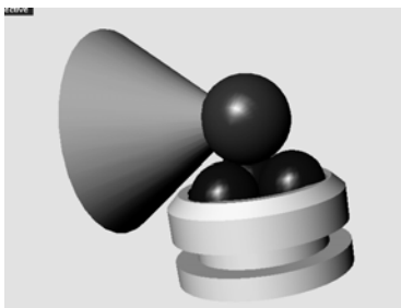
Fig. 1 Calibration ball sitting on a three point kinematic mount with the green cone representing the light from the transmission sphere focused at the center of the ball. The ball acts like a convex mirror and directs the light back into the interferometer over the same path that it exited.
